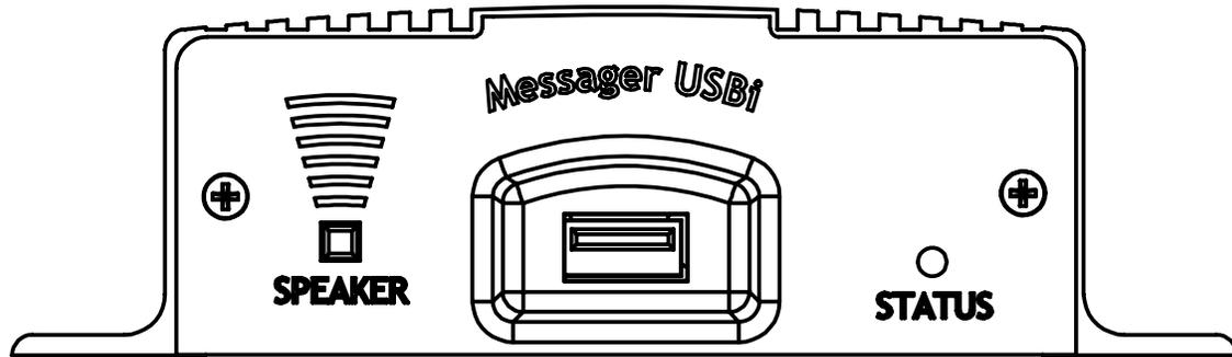
**SPEAKER** - The SPEAKER switch can be turned ON and OFF to monitor audio playback. The switch has no effect on the audio output connections on the rear of the unit. Switch should normally be kept OFF.
