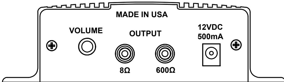
**VOLUME** - This pot is used to control the 8Ω and 600Ω output level of the stored messages. Volume up is clockwise, volume down is counter-clockwise.
